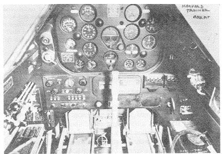
A Harvard cockpit; to the uninitiated "a hopeless collection of black faced dials and toggle switches." But having mastered the Harvard a pilot would feel at home in most every fighter aircraft for he would find the same instruments in the same place. (PMR 74-259)
